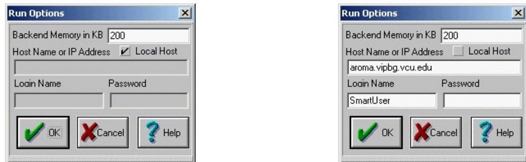
Figure 2.8 The Host Options Panel for local PC use (left) and remote Unix use (right).
